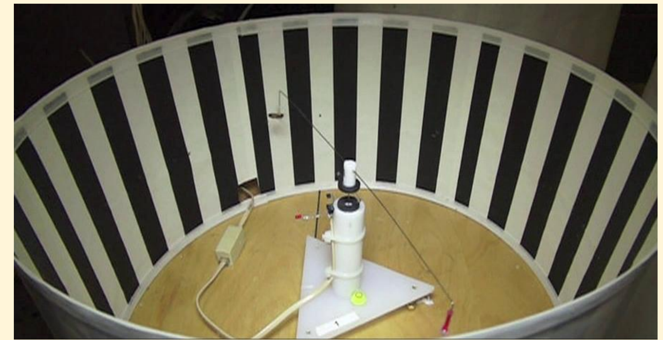
Figure 1. Flight mill used in the test, with a bee flying attached to one extremity (upper one) of the flight mill arm. Design based upon the plans of Teah Smith (WSU TFREC).
